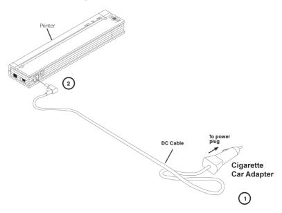
Figure 3. Connecting the printer to DC power
